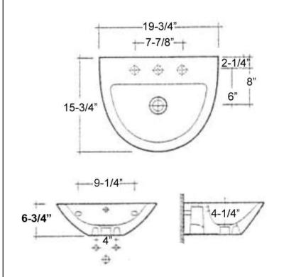
Dimensions of fixture are nominal and may vary within the range of tolerances established by ASME Standard A112.19.2. Dimensions and specifications subject to change without notice.
